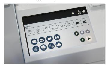
The DigiFold Pro 385 uses our patented flying knife technology which was developed to prevent the scuffing and marking on digital stocks that are caused by folding using conventional methods. This dispenses entirely with buckle plates and conventional knives, using instead an electronically controlled contoured flying knife around extra large diameter rollers and moving at the same speed as the material passing through the machine.
