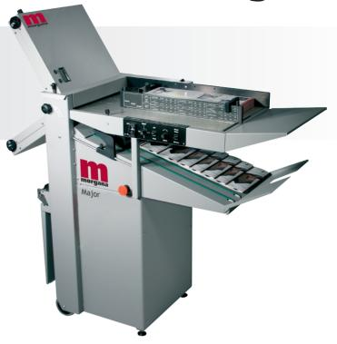
An optional rear delivery belt stacker is available for longer runs, when used with the roller bypass unit.
